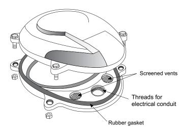
Figure 4-5, Examples of Standard Well Caps
