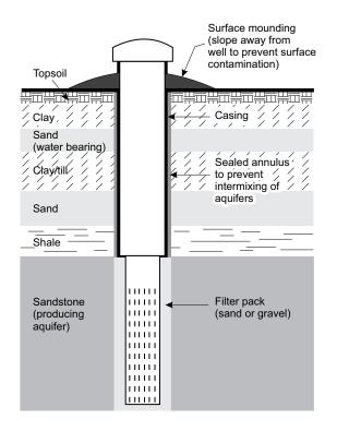
The annular seal will be disturbed during installation of the pitless adapter. It is the responsibility of the person completing this intallation to re-establish the annular seal back up to ground surface.
