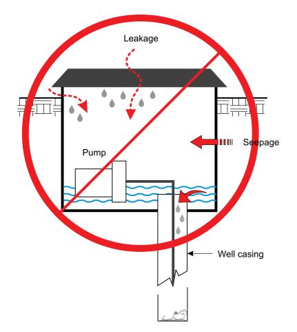
Well pits are "confined spaces" that can be a safety hazard to anyone who enters the pit. The air in the pit can become oxygen deficient or may contain dangerous gases that can come up from groundwater through the well. In Alberta, well pits have exploded due to the build-up of methane gas and people have died from asphyxiation after entering oxygen-depleted well pits.
