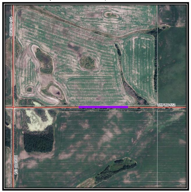
350M – of a Cut/Fill balance lowering the hill and backslopes with improvements to road grade in both directions to tie into existing road grade.
